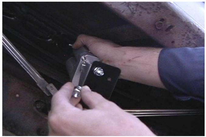
Note: Do not over tighten the actuator bolt, only tighten enough to compress the lock washer.
